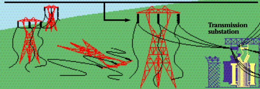
**Step 2.** A co-op may have several local distribution substations, each serving thousands of consumers. When a major outage occurs, the local distribution substations are checked first. A problem here could be caused by failure in the transmission system supplying the substation. If the problem can be corrected at the substation level, power may be restored to a large number of people.
